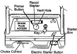
**CAUTION:** This starter is equipped to operate on 120 volt AC household current. Follow all instructions carefully as set forth in the "To Start Engine" section. When connecting 120 volt AC power cord, always connect the cord to the switch box on the engine first, then plug the other end into the household receptacle. When disconnecting the 120 volt AC power cord, always unplug from the household receptacle first.
